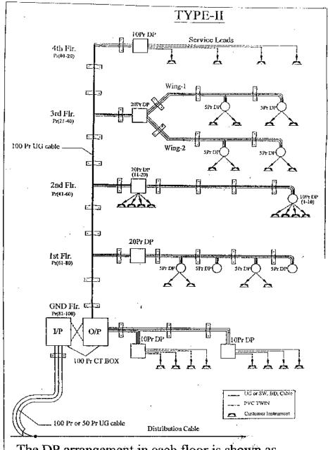
The DP arrangement in each floor is shown as suitable for different types of building structure.
